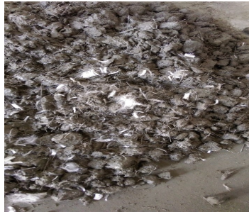
Figure 2: Addition of Glass Fibres with Cementitious Materials
